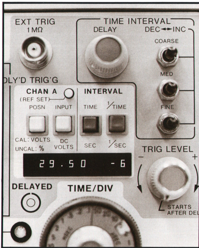
Fig. 5. The microprocessor is activated by pressing one of the function buttons (POSN, INPUT, TIME, 1/TIME). If any of the oscilloscope controls are not set appropriately for the measurement selected, the digital readout displays "0".
